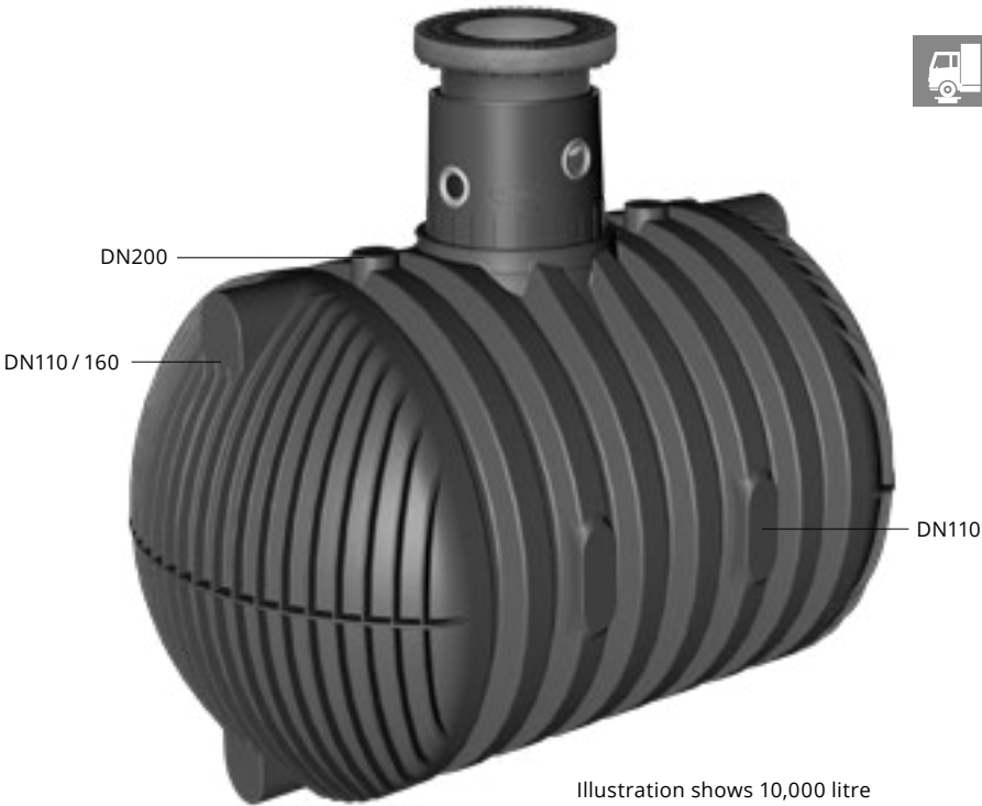
Illustration shows 10,000 litre tank with telescopic dome shaft 600 with cast iron lid, suitable for vehicle loading.
