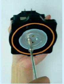
**HP-150/200** **REPLACING THE CHAMBER BLOCK**
