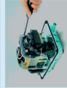
**HP-150/200** **REPLACING THE CHAMBER BLOCK**
