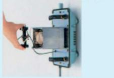
Install the SP switch to the frame with the screws.
