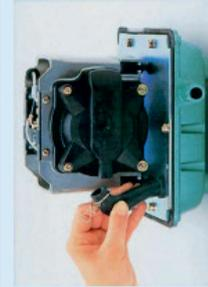
Pull out the L-tube from the casing block.
