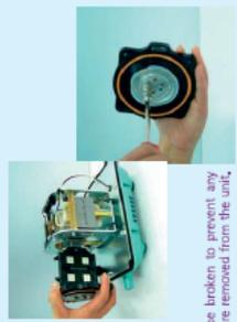
**STEP 6** **REPLACING THE DIAPHRAGM**
