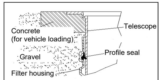
**Caution:** If the soft soap dries, the telescope becomes difficult to move and there is a risk that the seal may slip out of the seal groove. Before backfilling, the seal must be checked for a correct fit. The telescope must be sufficiently lined so that forces can under no circumstances be transferred to the housing.
