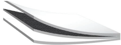
Figure 17: 3-ply layer structure
