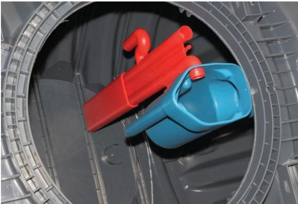
The sampling unit's outlet connector is placed into the outlet pipe's socket (use lubricant!). The socket connection should be secured with a Spax screw.
