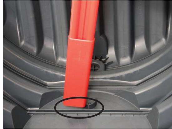
The lifter is placed from above to hold the dividing wall.
