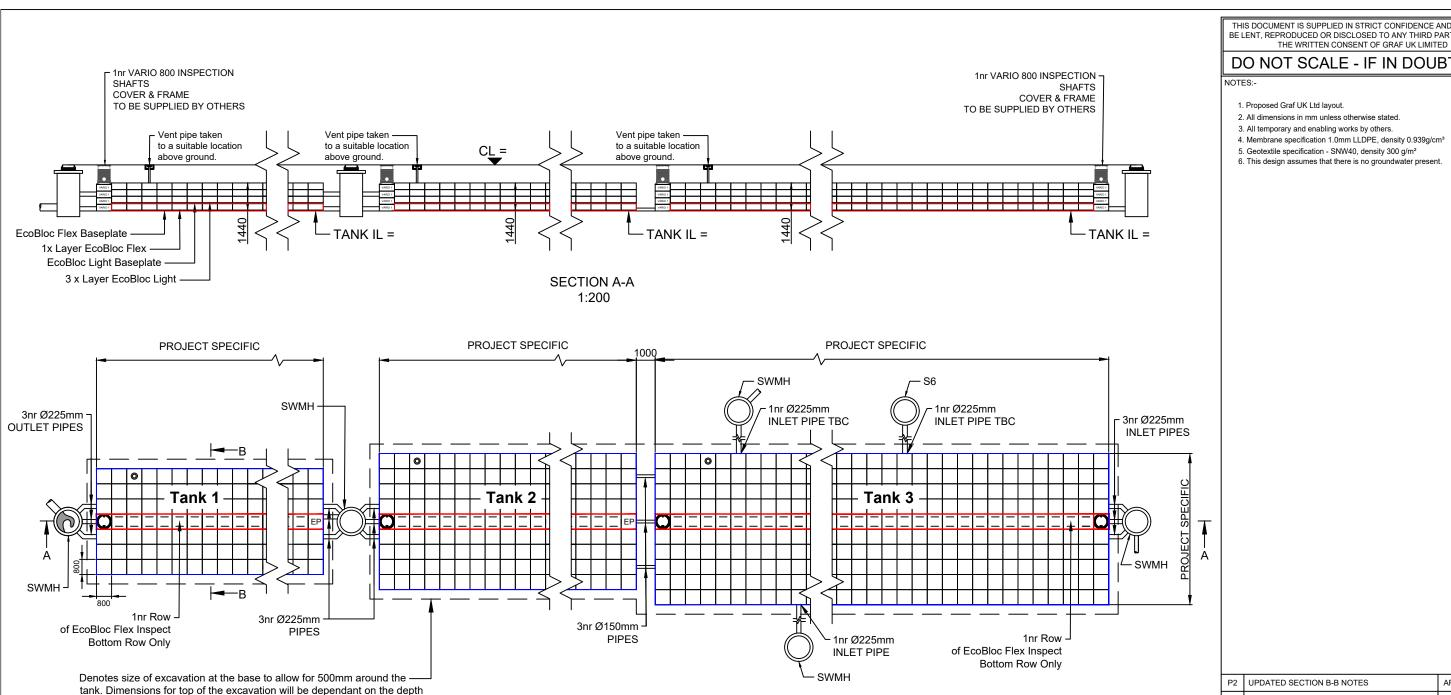
NOTE: EXCAVATION TO EXCEED TANK SIZE BY 500MM ON ALL SIDES TO ALLOW FOR ACCESS
