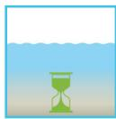
There is no aeration in the second phase. The activated sludge and the remaining settleable solids can now settle by gravity. A clear water zone is created at the top and a layer of mud forms at the bottom. Any floating sludge which might develop is located above the clear water zone.
