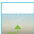
The wastewater is subjected directly to aerobic treatment for a fixed amount of time. On the one hand the microorganisms (activated sludge) are supplied with the oxygen necessary for degradation; on the other hand mixing is achieved as a result of pressure aeration. The air diffuser of the system is supplied with ambient air by a compressor. The aeration is intermittent, so as to allow targeted wastewater treatment. Thus, different environmental conditions can be achieved.
